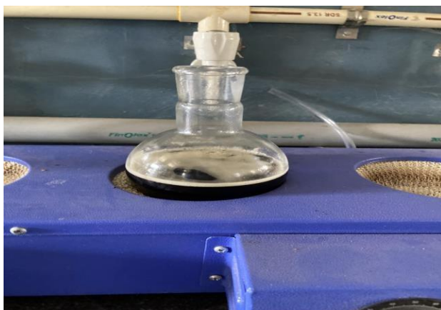
( Fig 1) preheating of jatropha oil
